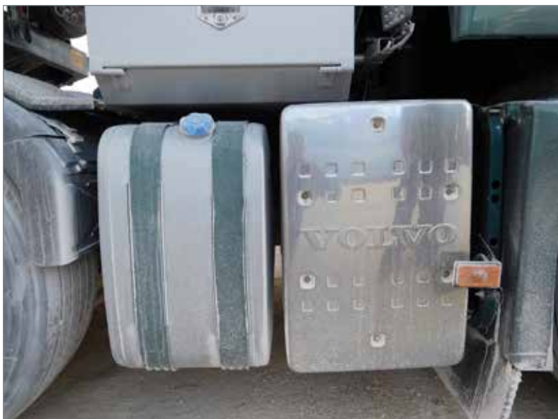
AdBlue® is stored in a dedicated tank and injected into the exhaust stream ahead of the SCR catalyst. Regular testing for contamination ensures that emissions are reduced.
