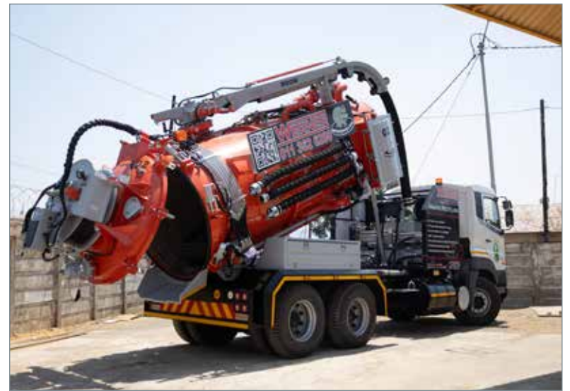
Werner Pumps' water-wise, truck-mounted recycling unit for municipal wastewater maintenance.
