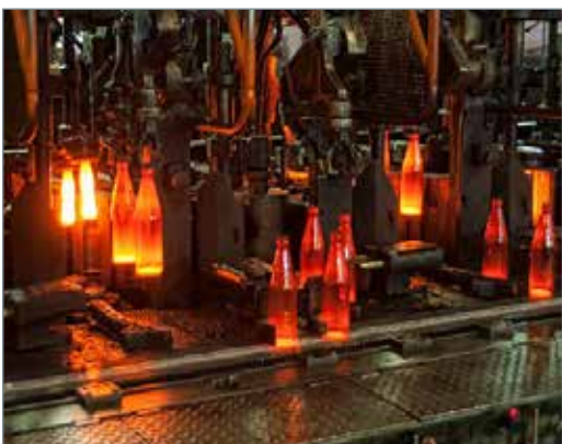
Knuckleback belts collect bottles from the furnace.
