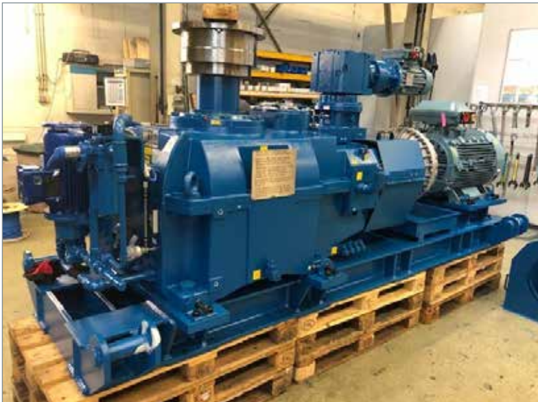
BMG supplies and supports the Sumitomo Hansen P4 range of Industrial Gear Units which has been engineered for Desolventiser Toaster, Dryer Cooler and combined Desolventiser-Toaster-Dryer-Cooler installations used in vegetable oil extraction plants.
