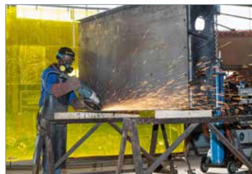
Factory work on a girder for one of the 50-ton, 20m-span Condra cranes.
