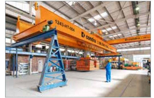
Factory testing of one of the four 50-ton, 20m-span cranes for Zambia. This particular crane also features a 10-ton auxiliary hoist.
