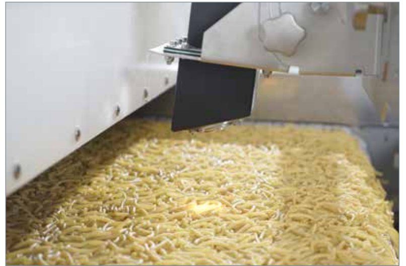
The Bühler PastaSense in-line quality monitoring system for industrial pasta production.
