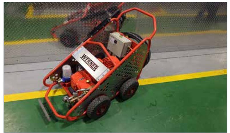
One of Werner Pumps’ redesigned industrial high-pressure washers built with a “racing-car” style cart that boosts manoeuvrability, stability and on-site safety.
