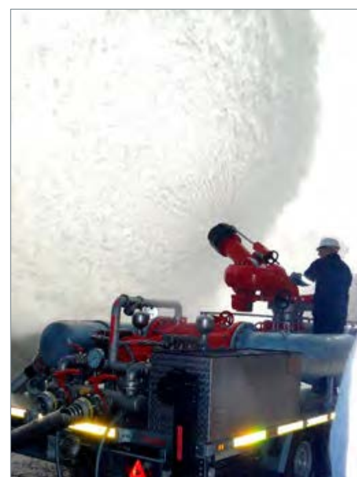
Latest firefighting technology arrives in South Africa, FireDos foam dosing and monitor trailer flow in water wall / fog pattern at 18,000L/min.
