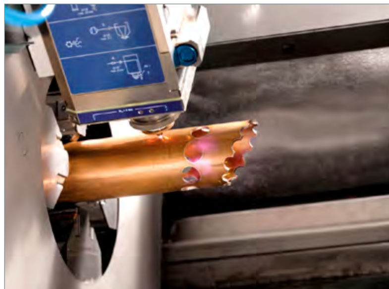
BLM fibre laser machines can cut to length, drill any size hole or cut any shape geometry - all in a single machine.
