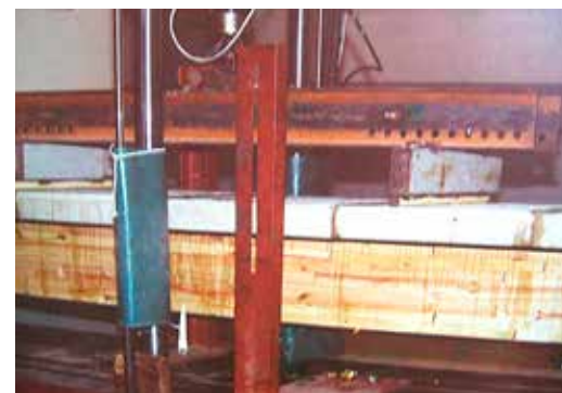
Machine testing for grade verification.
