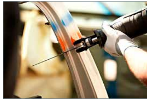
Robust and durable for the toughest applications, these saw blades have sharp carbide teeth welded onto them.
