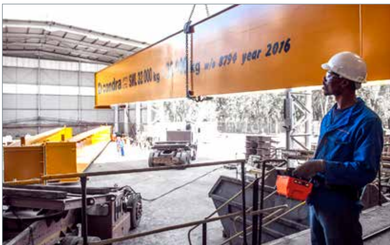
Foreground: Part of one girder leaving Condra's factory; Background: Two completed girders with road transport standing by. All girders are part of the two 60 ton portal cranes ordered by Stefanutti Stocks for its pre-cast yard in Port Elizabeth.
