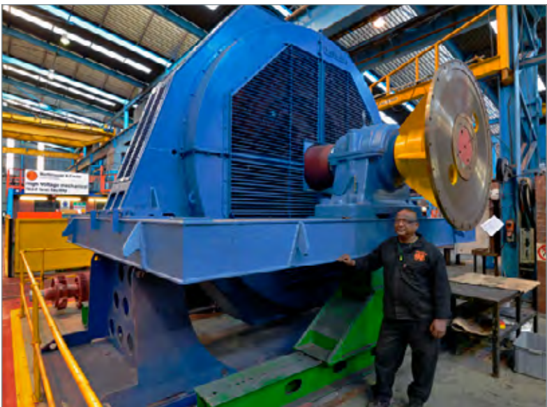
Marthinusen & Coutts's test technician, Suresh Gunpat, with the 40 pole synchronous mill motor during the series of tests conducted on it on completion of the rehabilitation process.
