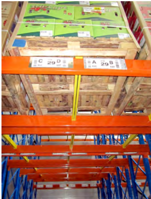
Pallet Support Beams are important, as most South African fruit pallets are disposable.
