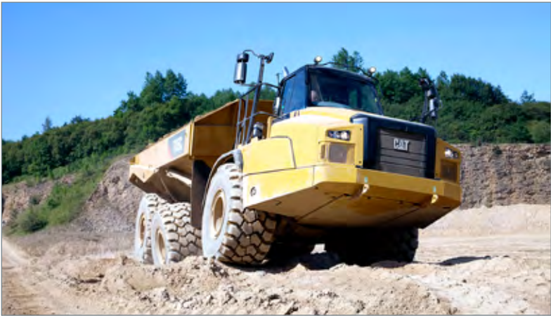
The Cat 745C has a newly designed dump body with a capacity (heaped SAE 2:1) of 25m 3 and an increased payload of 41 tons.
