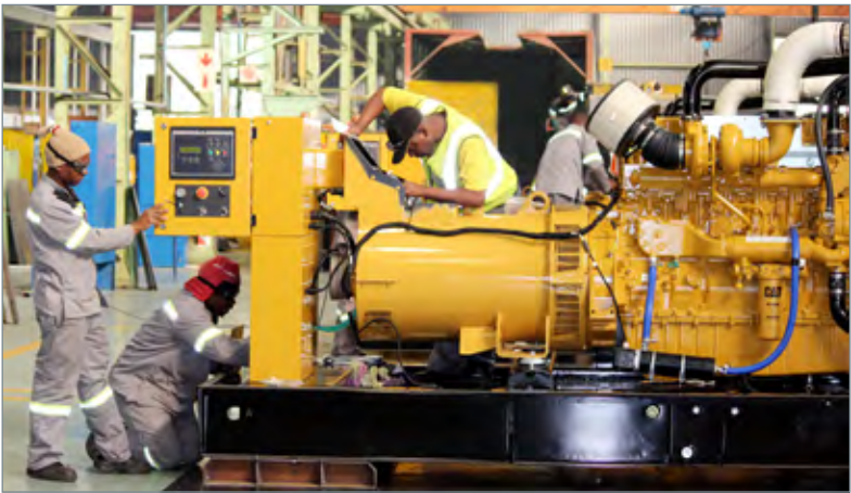
A significant milestone is reached as a 550kVA Cat C15 diesel generator set is assembled at Barloworld Power’s Boksburg facility.
