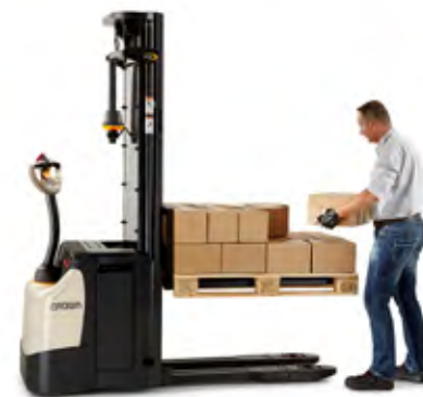
Crown has extended its tried-and-tested QuickPick Remote technology with a variant that controls lift and lower functions.
