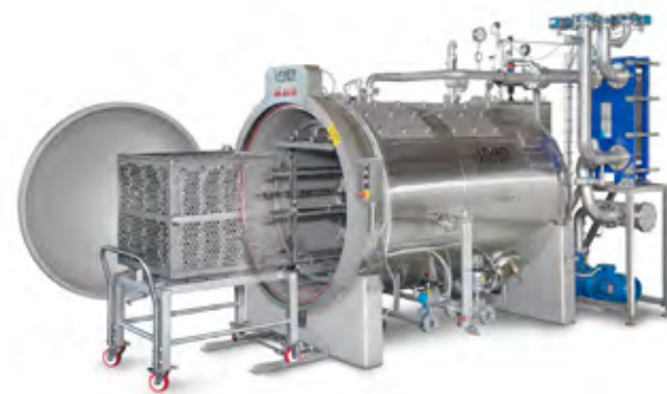
The Levati Rotary Retort uses an enhanced spray sterilisation with both fixed and rotating nozzles that offer improved heat distribution and penetration across loaded baskets.
