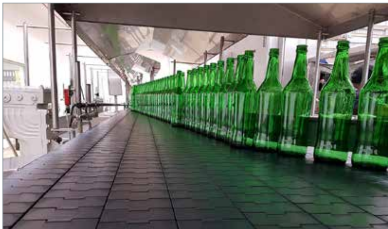
BMG's new range of dry running conveyor components for the food and beverage sector.
