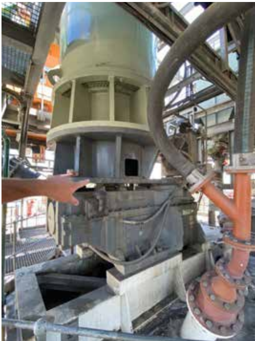
An example of the new standard flange mount electric motor which will not fit onto this gearbox, so motor dimensions have to be modified, usually with an adaptor plate.
