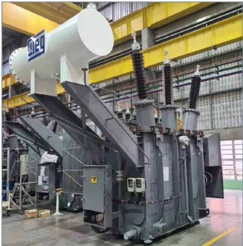
One of the eight WEG 6MVA traction transformers.
