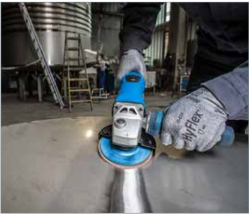
Dressing a stainless steel weld with a PFERD POLIFAN CO-FREEZE INOX flap disc.
