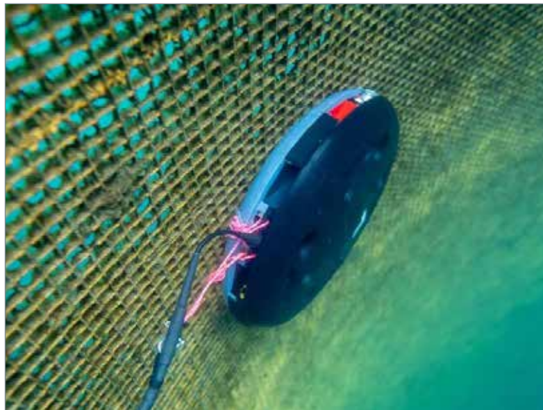
The Probot drone uses a preventive method that cleans the nets and prevents biofilm creation © Probotic
