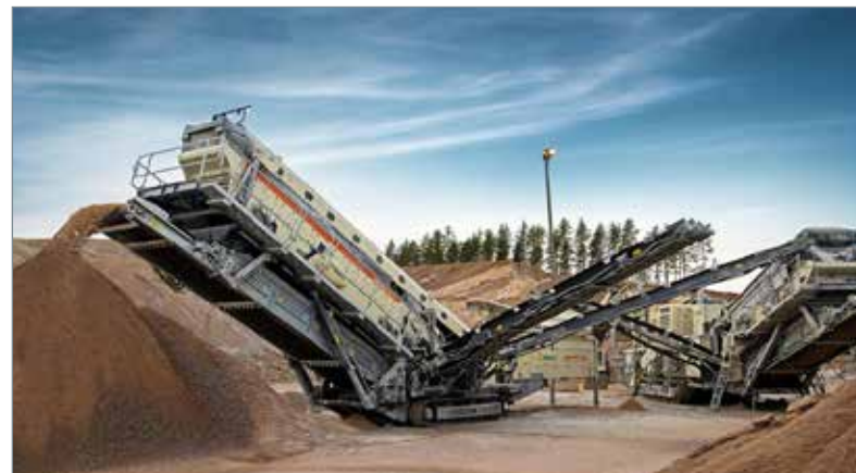
The Lokotrack ST4.10 features a large 6m x 1.5m screen box which is rated to handle up to 600tph.
