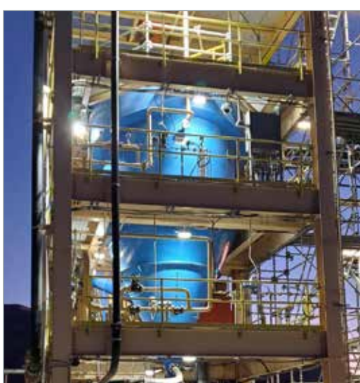
Using a novel aeration system to disperse fine bubbles into a fluidized-bed environment, the HydroFloat® Separator significantly increases the selective recovery of coarse particles by applying flotation fundamentals to gravity separation.
