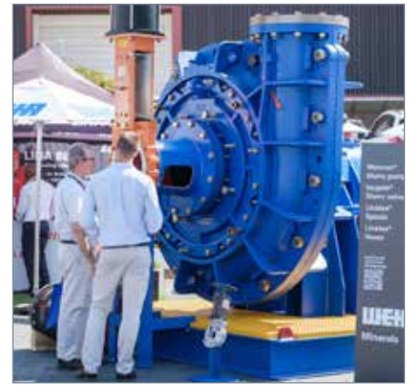
A Warman MCR400 connected to a Linatex rubber lined spool and Isogate WS 400 knife gate valve.
