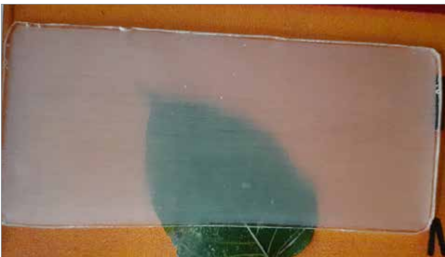
Transparent wood may be a sustainable alternative for glass or plastic used for making windshields, see-through packaging and biomedical devices. Credit: Anish M. Chathoth
