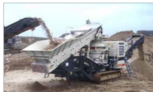
The Lokotrack® LT300HP™ features the most popular Nordberg® HP300™ cone crushing unit, which provides optimized performance, efficiency and high capacity in crushing.
