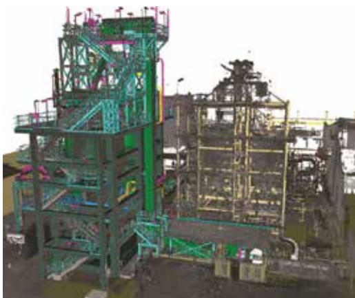
A salt dissolving plant – a typical application of 3D scanning.
