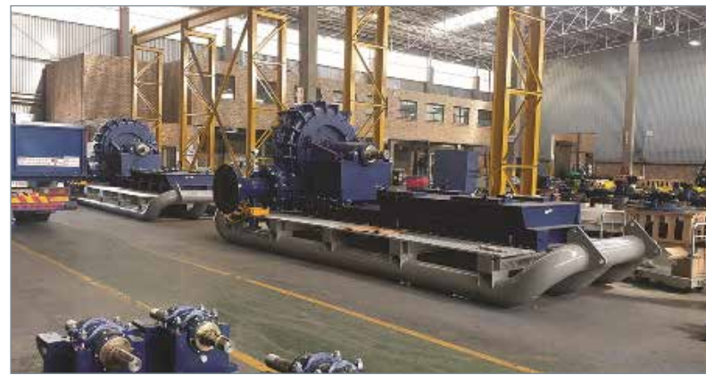
A KREBS® slurryMAX™ high pressure tailings pump on a mobile skid.
