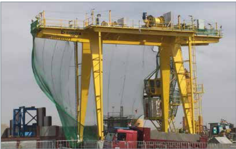
Condra's 25-ton pre-sink portal cranes, on site at a mine in Asia during the shaft-sinking phase.
