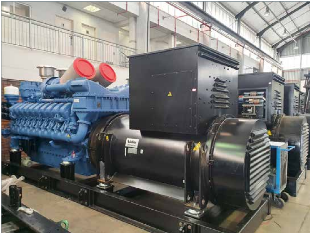
3000kVA 400V primary equipment prior to enclosure installation.
