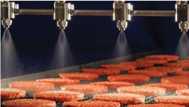
Monitor Engineering's antimicrobial spray system for meat applications.
