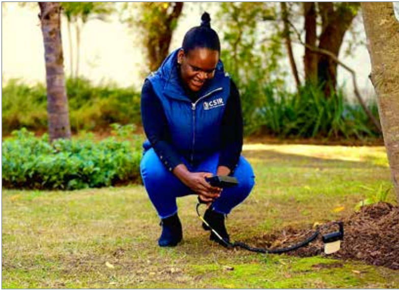
Dr Mpumi Mobe, senior researcher at the CSIR using a handheld Hydro-Sense II system to measure volumetric water content of soil.
