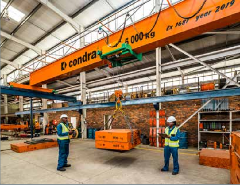
Typical single-girder overhead crane under test in Condra's Johannesburg factory
