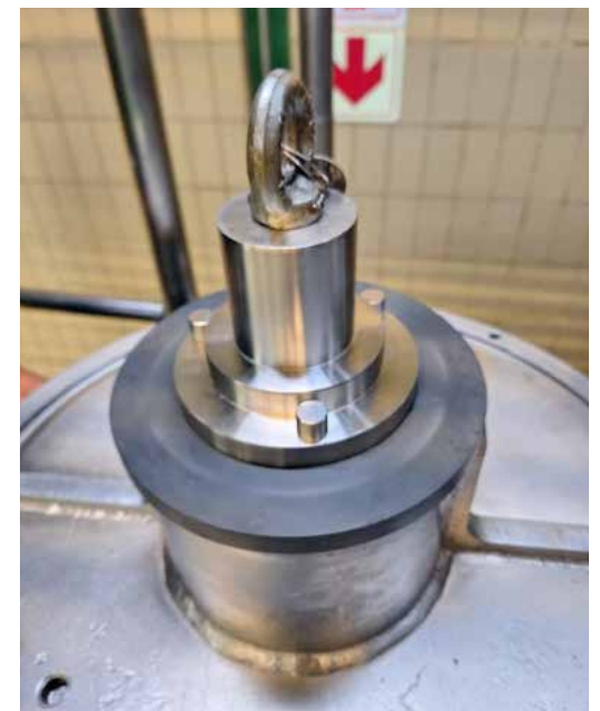
A Vesconite thrust washer has been successfully employed on a grinding machine at a large fruit juice concentrate producer.
