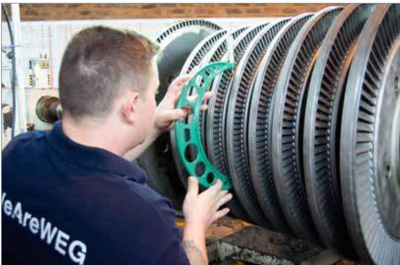
Measuring of labyrinth seals on a turbine rotor.
