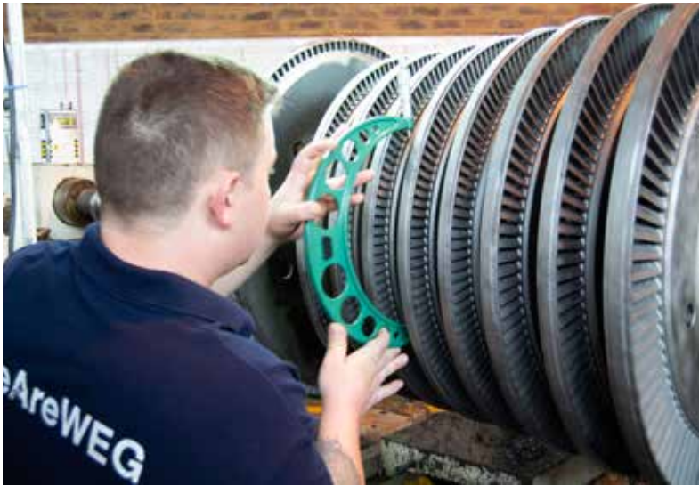
Measuring of labyrinth seals on a turbine rotor.
