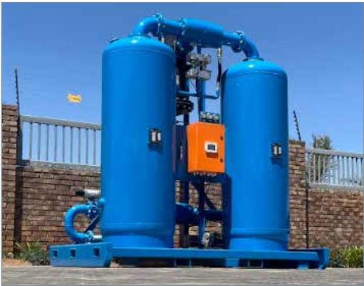
A heatless SA 5580 desiccant air dryer constructed by Artic Driers with a capacity 95 m 3 /min at 7 bar with a dewpoint of minus 40°C.
