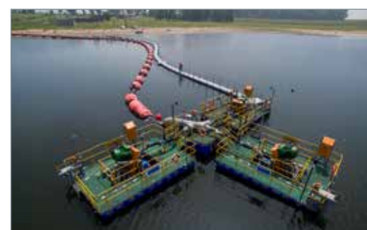
Weir's pontoon solution is useful for emptying holding dams where it can draw water from the middle of a dam.
