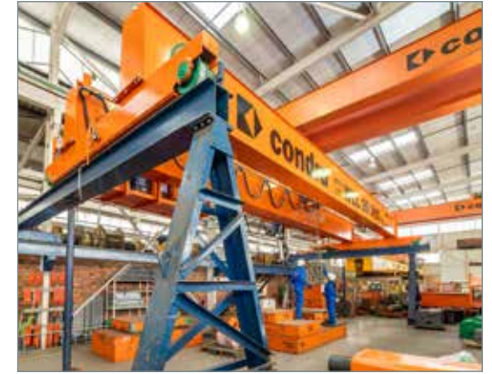
Typical double-girder overhead crane under manufacture in Condra's Germiston factory.
