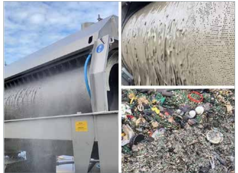
The Lackeby Roto-Sieve® RSS24 drum screen separates impurities from oil. Photo courtesy of TASK Environmental Engineering.
