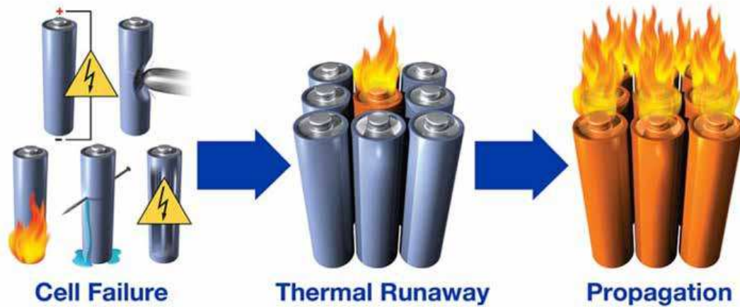
A schematic showing how a lithium-ion battery fire develops.
