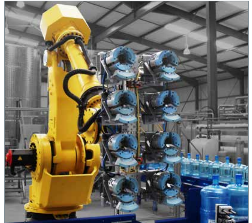
A robotic handling system capable of lifting and placing eight 20-litre water bottles simultaneously during the automated refilling process, enabling high-speed, consistent material movement.
